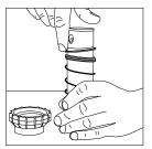
Carefully work the new flexible rubber seal, flat side up, onto the nozzle turret, and then down onto the riser body. Take special care not to twist or deform the flexible
