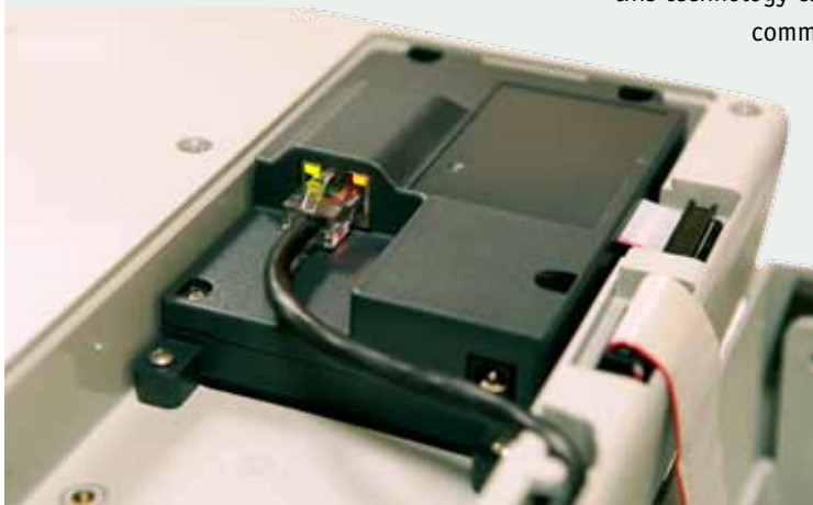
ACC-COM-LAN: features a standard network jack on the back for easy connection to a customer's computer network.
