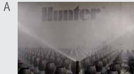
Sprinklers undergo testing in the Precipitation Analysis Lab.
