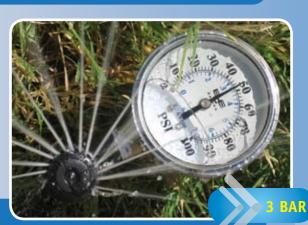
The Solution: Lower flow rotators provide improved dynamic system pressure from 1 Bar to over 3 Bar resulting in healthier lawns.
