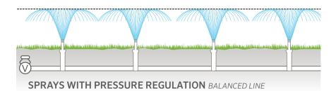
When designing with the pressure-regulated Pro-Spray PRS40 Sprinkler Body, each head will precisely regulate to 40 PSI, the optimal pressure for the MP Rotator Nozzle.
