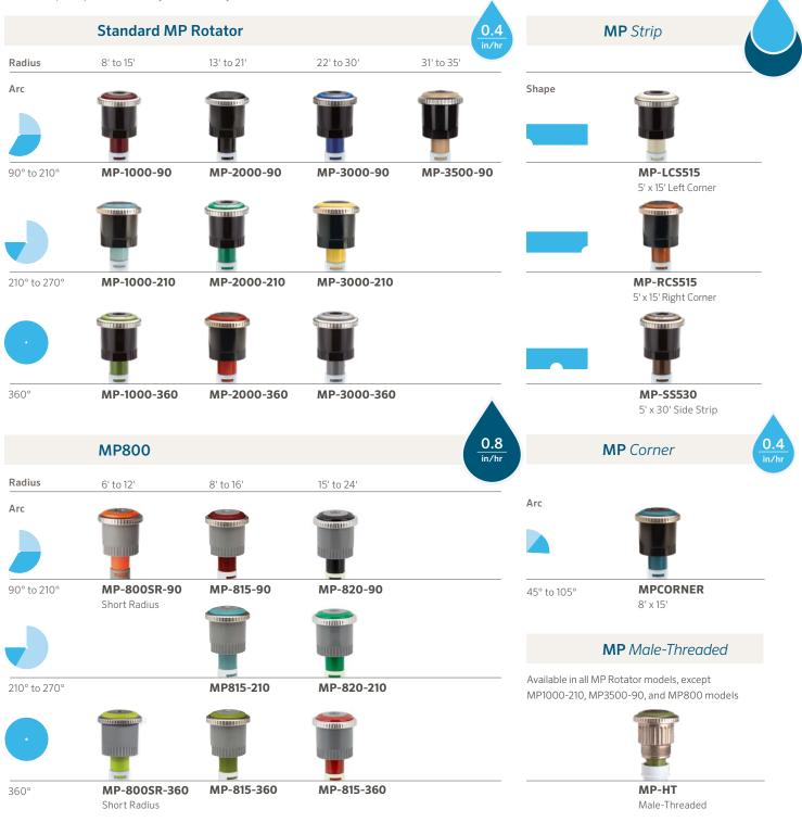
Note: The MP800 has a precipitation rate of 0.8 in/hr. Since this precipitation rate differs from the Standard MP Rotator rate of 0.4 in/hr, we recommend zoning the MP800 separately to maintain matched precipitation within each zone. MP Strips can be used with both the Standard MP Rotator and the MP800, depending on the layout.
