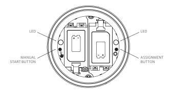
To enter Assignment Mode, press and hold the right button inside the WVL battery compartment for 2 seconds until the right (gear) LED lights up yellow.
