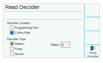
The menu will now allow selection of Station, Pump, or Sensor decoder types. Select the type of decoder to re-program, then enter the address. Press Read Decoder to get the current setup for item you selected, then enter the changes. Press Program Decoder to send the changes down the two-wire path to the selected decoder.
