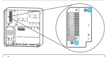
Do not attempt to connect the facepack cable to this port. The connector has a protective cover that should be left in place until the connection is needed.
