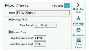
Each Flow Zone has a check box for "Manage Flow" and "Monitor Flow." To monitor flow, check that box. Then complete the settings and rules for the Flow Zone.
