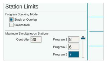
Maximum Simultaneous Stations sets a hard limit on the number of stations the controller can run at once, regardless of Flow Manager or other settings. The ACC2 Decoder controller can run approximately 20 Hunter solenoids at once on a single output module, including P/MV outputs. The decoder controller can run up to 30 stations at once, provided they are spread over multiple decoder output modules, with not more than 20 active on each output module.
