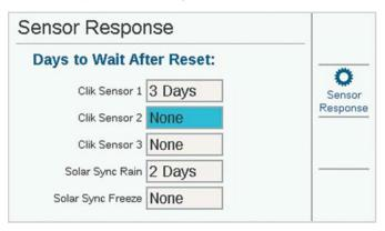
**Rain Delay:** In the Sensor Response menu, press the soft key for Rain Delay. This optional setting will cause watering to stay off for a set number of days, after the sensor activation is over. Select the number of days for watering to stay off for each Clik sensor input.
