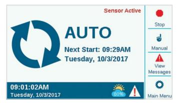
If Solar Sync<sup>®</sup> is installed and enabled (**Devices** menu), the Solar Sync symbol shows the current adjustment percentage in the lower right of the border.
