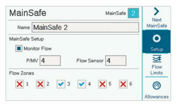
MainSafe zones generally require their own flow sensor, and their own Master Valve. Often these are Normally Open Master Valves, which only close in the event of an alarm.
