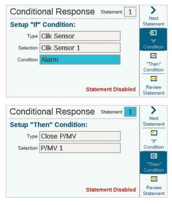
Clik Sensors can use alarms as a trigger. They can also trigger based strictly on their position, Closed or Open, without causing an alarm.
