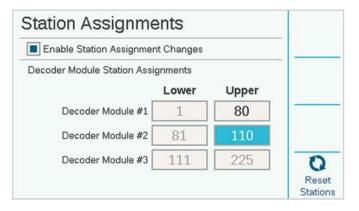
Each output module provides 75 stations when it is installed. If you need more than 75 stations on a single two-wire path, or on paths from a single module, you can reassign the station numbers from the other module(s) to the first module, and so on.
