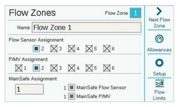
Flow Sensor Assignment: Check the box for the Flow Sensor or sensors connected to the Flow Zone.
