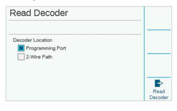
Then press the soft key labeled Read Decoder. This will return the configuration of the decoder in the port, with a screen for entering the station numbers. If the screen says "Decoder Not Found!" the decoder wires may be disconnected, or the wrong wires may have been inserted.
