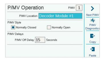
All P/MV outputs are set to Normally Closed operation, but they can be changed to Normally Open functions in the Devices menu. See P/MV Operation section on page 20.
