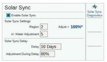
**Solar Sync Delay** allows a number of days to wait before automatic Solar Sync adjustment goes into effect (to establish new landscape, for example). Enter a number of days (1-250) to wait, and specify the **Adjustment During Delay** percentage to use during the delay period. At the end of the delay, the Solar Sync will begin adjusting automatically for the current climate conditions.
