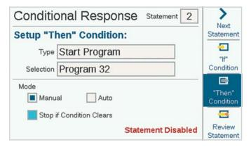
If **Stop if Condition Clears** is checked, the Station, Block, or Program will only run while the trigger condition is present. If the condition continues, a Station or Block will run for the specified run time, and a program will run once for the duration of the program.
