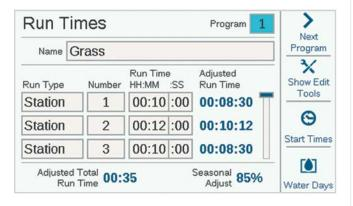
Verify that you are in the correct program, by number or name. Select the Run Type field, and select Station or Block ("Blocks" are described in detail in the Stations Menu section. Blocks replace "SSGs" in the original ACC Controller). Press the dial to select the type.
