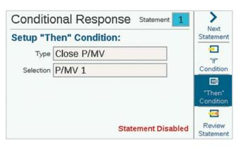
Clik Sensors can use alarms as a trigger. They can also trigger based strictly on their position, Closed or Open, without causing an alarm.
