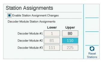
Each output module provides 75 stations when it is installed. If you need more than 75 stations on a single two-wire path, or on paths from a single module, you can reassign the station numbers from the other module(s) to the first module, and so on.
