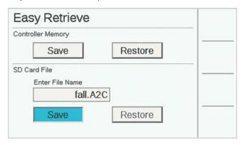
**Controller Memory:** Only one setup may be saved in Controller Memory, and it will remain unless you make changes and create a new Easy Retrieve backup in the future. You can choose Restore at any time, and it will change the whole controller to the last Easy Retrieve backup.
