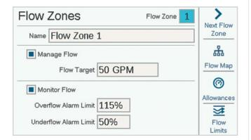
Each Flow Zone has a check box for "Manage Flow" and "Monitor Flow." To monitor flow, check that box. Then complete the settings and rules for the Flow Zone.
