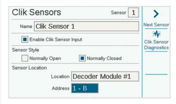
The controller sensor inputs are already configured as Normally Closed, but this can be changed for other types of contact-closure sensor inputs to Normally Open.
