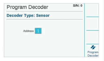
Select the sensor decoder address, and press the Program Decoder soft key to program the decoder. Mark the decoder and install at the sensor location.
