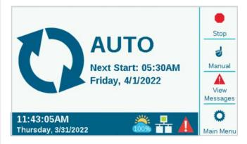
If a Solar Sync Sensor is installed and enabled (**Devices** menu), the Solar Sync symbol shows the current adjustment percentage in the lower right of the border.
