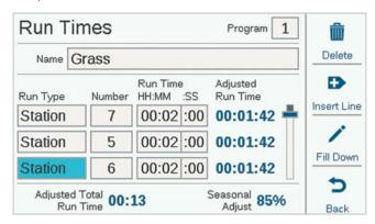
You can also **Insert** an item above any selected line in the list. Scroll to an item, and press Insert Line, and a blank line will appear above it.
