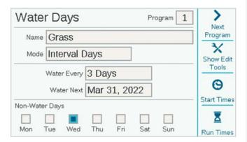
Both Odd/Even and Interval also have Non-Water Days, which can set a day (for example, a mowing day) on which watering will never occur, regardless of the schedule.
