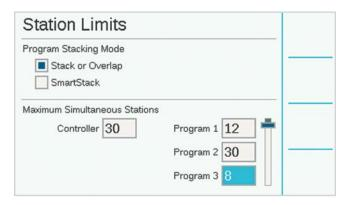
**Stack or Overlap** means that each program can be manually set to Overlap with other programs, or be required to stack. Programs that are set to stack can only run by themselves.
