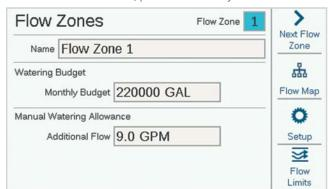
**Watering Budget:** Enter the total amount of flow that can be allowed in this Flow Zone in the calendar month. If the total flow exceeds the monthly budget, an alarm message will appear on the screen. The controller will not automatically stop watering when this alarm occurs.
