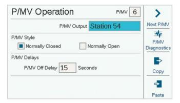
All P/MV outputs are set to Normally Closed operation, but they can be changed to Normally Open functions in the Devices menu. See the P/MV Operation section on page 20.
