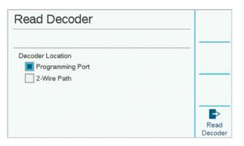
Then press the soft key labelled Read Decoder. This will return the configuration of the decoder in the port, with a screen for entering the station numbers. If the screen says "Decoder Not Found!" the decoder wires may be disconnected, or the wrong wires may have been inserted.
