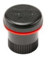
Brand: Residential & Commercial Irrigation Product Line: Nozzles Product Model: Bubblers & Bubbler Nozzles SKU: PCN10 Description: Pressure-Compensating Bubbler Nozzle, flood pattern, 3.8 l/min, female thread Weight: 0.01701 UPC-A: 0611698112472 Qty. / Bag: 25/250 Master Carton: 250 Land Pallet: 40000 Ocean Pallet: 48000 Application Type: Trees and shrubs Nozzle Type: Bubbler Fixed Arc Spec Nozzle Type: ½" threaded bubbler
