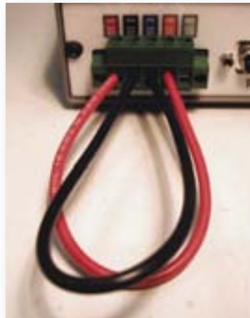
Figure 7: CCC Loop Back Wiring
