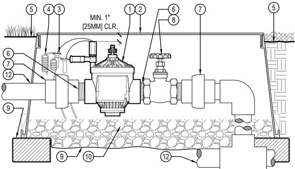
IN-LINE VALVE (PGV-201)WITH ACCU-SYNC, UNIONS AND ISOLATION VALVE
