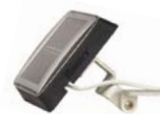
SPNODE Solar Panel Kit (optional) Height: 3¼" Length: 3" Width: 5⁄8" Controller to solar panel: 100' maximum 18 AWG direct-burial wire
